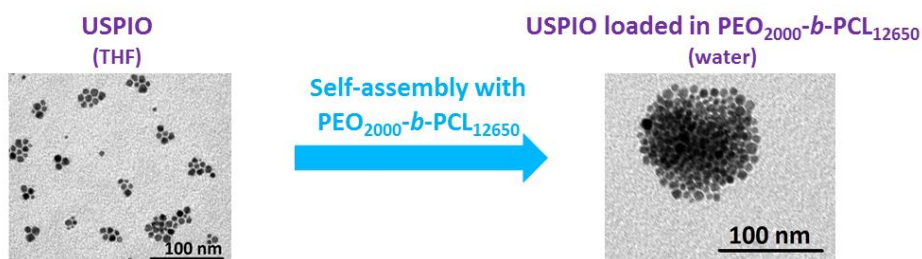
Figure 1. Clustering of USPIO into well-defined PEO 2000 - b -PCL 12650 nano-assemblies
