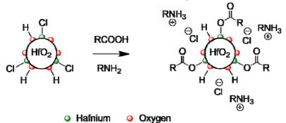
Scheme 1: Surface reaction from charge stabilized to sterically stabilized particles
