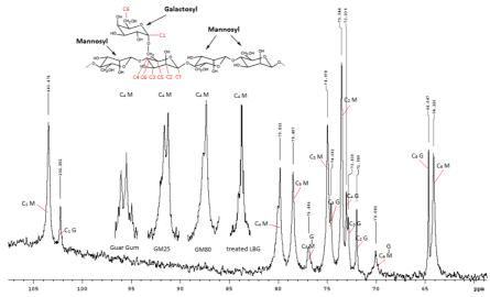
Fig. 1: [13C]-NMR spectrum of GM80 and superimposed mannosyl C4 signals of different galactomannans.
