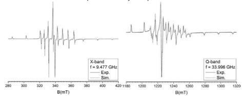
Figure 2 - X and Q-band spectra of V-doped MIL-53 at RT
