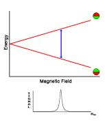
Continuous irradiation of mw Fixed microwave frequency Vary magnetic field Detection of absorption of mw
