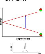
Continuous irradiation of mw Fixed microwave frequency Vary magnetic field Detection of absorption of mw FT-EPR
