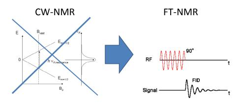
Continuous irradiation of mw Fixed magnetic field Vary rf Detection of absorption of rf
