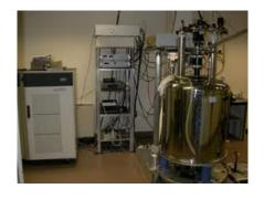
W-band - 95 GHz Cryo magnet Sweep from 0 to 6Tesla
