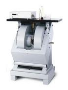
X-band - 9.5 GHz Water-cooled electromagnet Sweep from 0 to 1.4 Tesla
